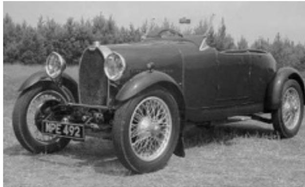
sixteen valve engines. These were lightweight high performance cars fitted various body types, racing sports and touring. From 1926 the lightweight cars on offer were the Type 37 and 37A sports (See details in Mainly for Fun Part Two) and the **Type 40 tourer**. Fitted with a 1496cc twelve valve single overhead camshaft four-cylinder engine, the 37A being supercharged. These were available to 1930.
