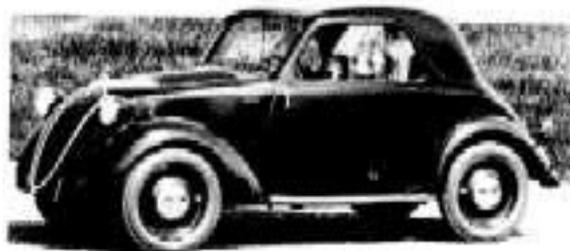
Giacosa's next design was the **Fiat 508C**. A completely new car to replace the 508, the 508C or as it became known as the "Millecento", had a 1100cc short stroke engine, with overhead valves, (The 500 engine had side valves), an outstanding chassis design that earned it a reputation for good handling and ride quality. It was with a 508C chassis that as engineering manager Danti Giacosa led a team that developed the **Fiat 508CMM** a streamlined coupe. Fiat used the car to win the
