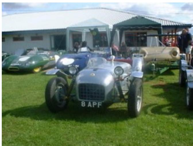
The **Lotus Mark 6**, sold in kit form is a good representative of the earliest cars produced by Chapman in the early 1950s, with a multi-tubular chassis clothed in aluminium panels. Engines fitted ranged from the 1172cc side valve Ford unit to the then new 1100 cc Coventry Climax engine. For most of the 1950s Lotus concentrated on producing bespoke sports racing cars. The Mark 6, Mark 8, Mark9, Mark 10 and the Eleven models. In 1957 Chapman's introduced a couple of new light car designs .
