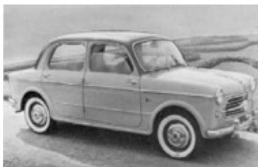
His next light car design was the **1100-103**; this model perpetuated the name Millecento previously given to the 508C. This Millicento was a compact unitary construction saloon fitted with wishbones and coil springs at the front and a live axle and half-elliptic springs at the rear. Its excellent handling
