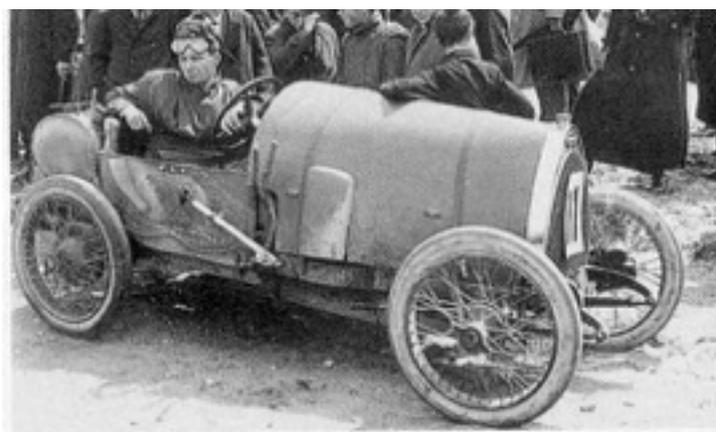
Ettore Bugatti famous for his grand prix and luxury cars always worked to a high standard of refinement. In 1910, the first of his designs bearing his name to be offered to the public. With a 1327cc single overhead camshaft eight valve four-cylinder engine fitted. It was available with three wheelbase lengths, the **Type 13** the shortest and the Type 15 and 17 longer to suit body types.
