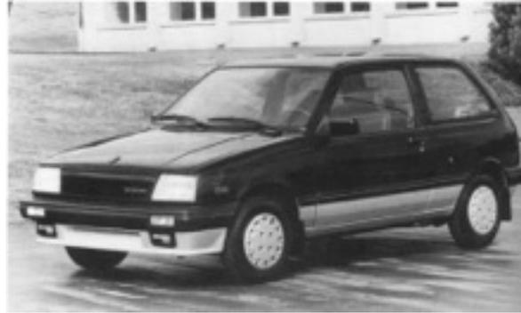
The Suzuki SA310 was a front wheel drive car and had a 993 cc three cylinder overhead camshaft engine. It was assembled in seven countries around the world and sold with many names such as **Suzuki Swift**, Cultus, Khyber, Forsa, Holden Barina in Australia, Chevrolet Sprint/Sprint Metro, Pontiac Firefly in Canada, Isuzu Geminett in Japan and was in production from 1983 to 1988 in its first version.
