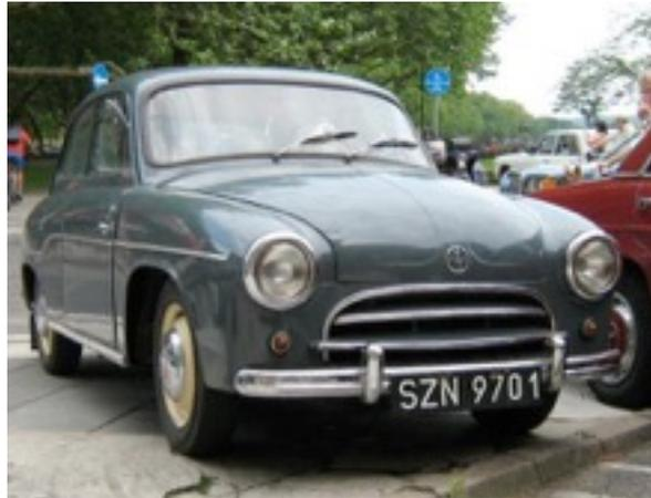
The last of the European three cylinder two-stroke engine cars was the Polish produced **FSO Syrena 104**. The original Syrena had been produced with twin-cylinder since 1960 and in 1966 an updated model that had a three-cylinder two-stroke engine with a capacity of 843 cc that was also later produced by FSM in Warsaw. Between then they produced over half a million Syrena by 1983. By then the two-stroke triple had been adopted by the Japanese motor industry.
