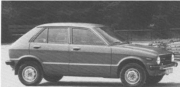
The first of a new breed was the 1977 **Daihatsu Charade**, fitted with the first of the CB series engines, the CB10 of 993cc. The Daihatsu Charade was a new front wheel drive model with a new three-cylinder belt driven overhead camshaft engine the Daihatsu C series engine of 843 cc or 993 cc. Japanese Car of the Year in 1979 and was made with successive revisions from 1977 to 1993. It was assembled from kits in many countries around the world.
